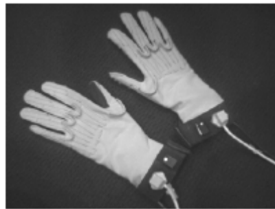
Figure 2. CyberGlove with Polhemus positioning receivers mounted.
