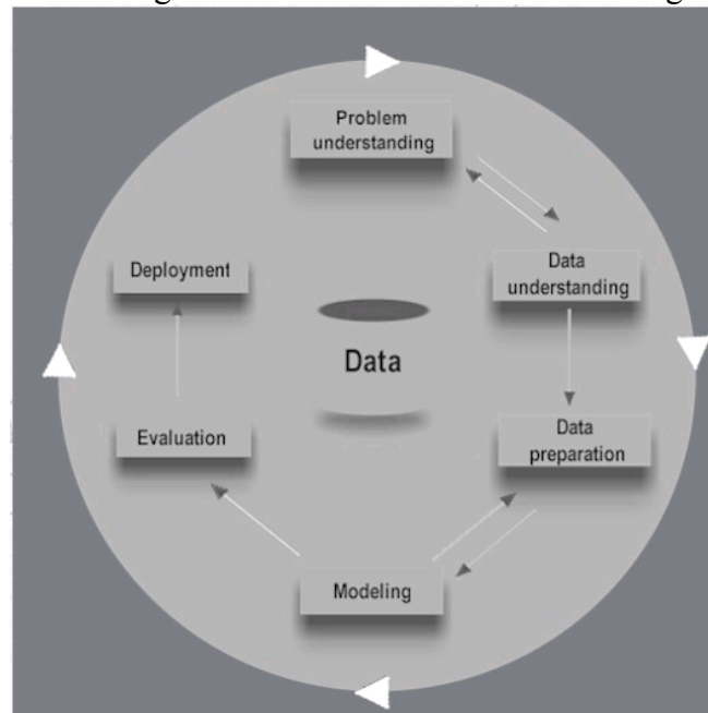
Figure 1. Basic flow of data mining process (Gamberger, Šmuc and Marić, 2001)
