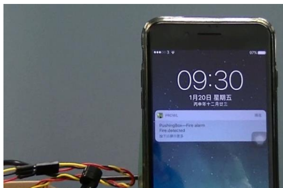
Figure 4. The Modified Fire Alarm System Sending Push Message to a Mobile Phone.
